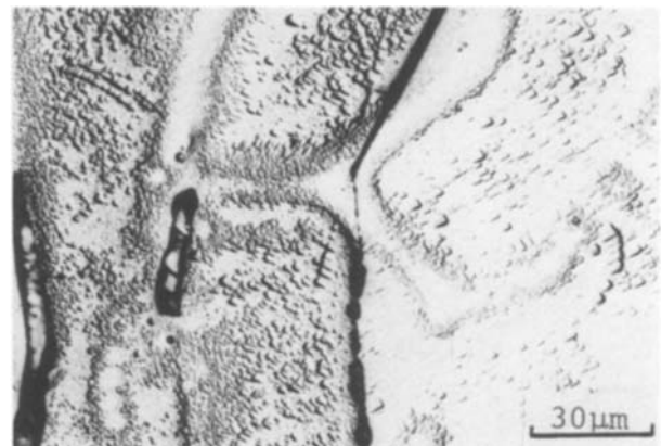
Figure 14 Micrograph of Sample 22 showing etch pits which belong to two differently orientated grains. Each grain has subgrain boundaries.
